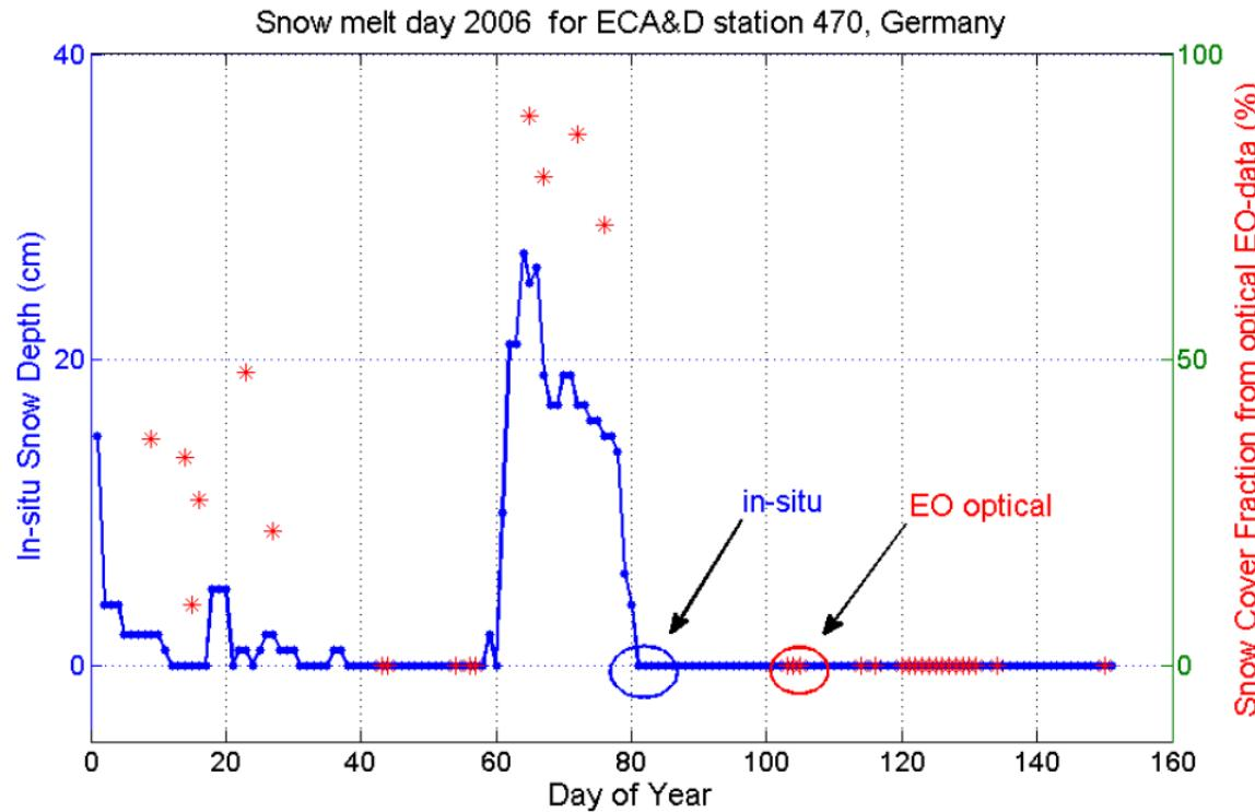
Fig. EO vs. in-situ observation of snow. Fig by S. Metsämäki
